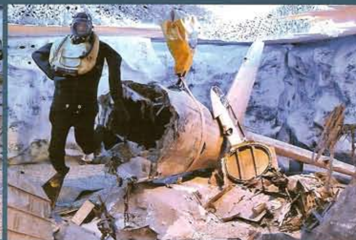
On display at the Fleet Air Arm Museum, Yeovilton, UK is the substantial remains of Skua L2490 which was also recovered from Norway in 1974, from Lake Breidal. The aircraft had sunk into the frozen lake following an attempt to destroy it by setting fire to the cockpit following a forced landing.
